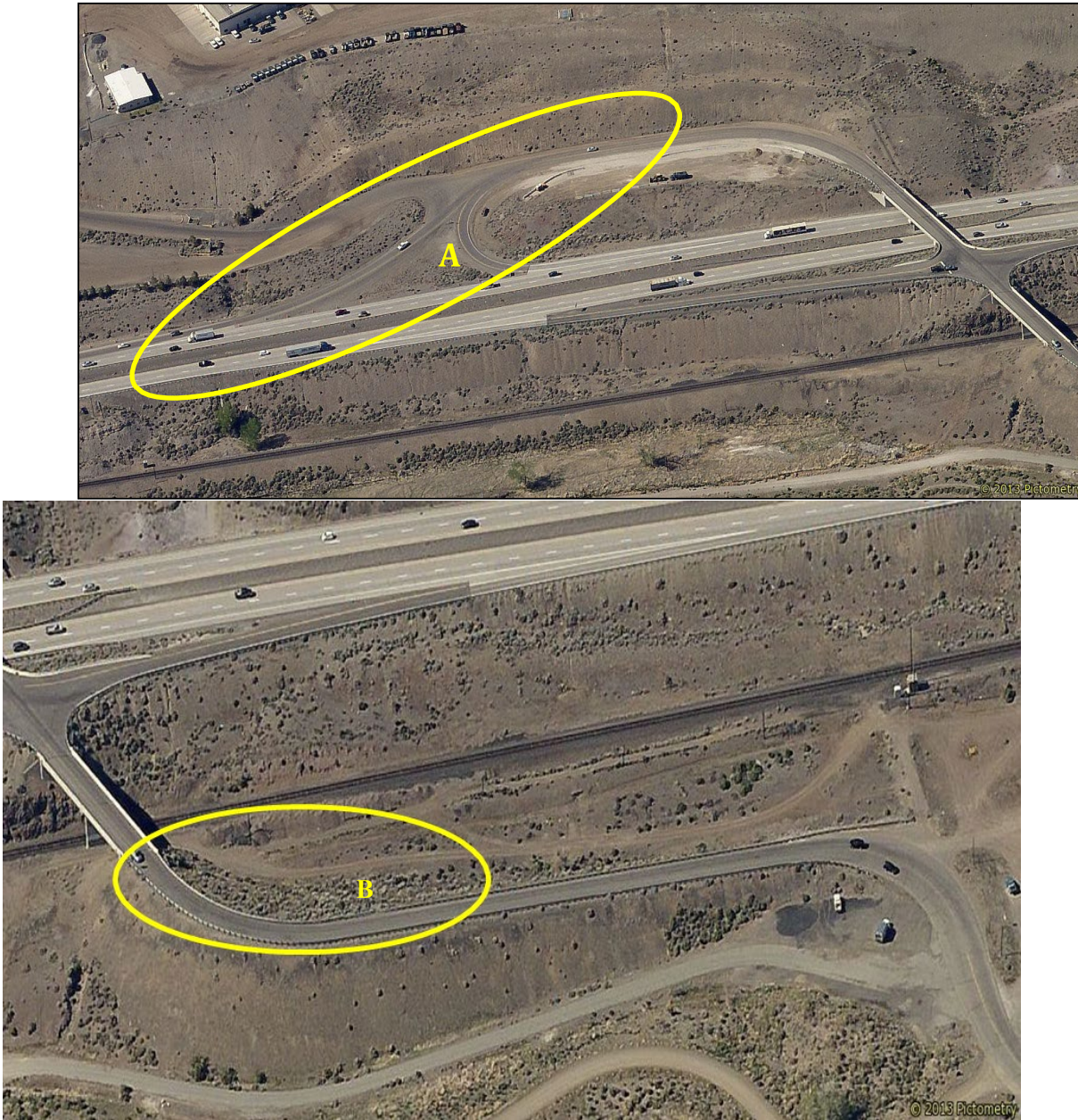
Figure 3.4-35: Existing Infrastructure Connecting Lockwood to Interstate 80. “A” and “B” denote areas with substandard traffic flow for entering and exiting Interstate 80.
